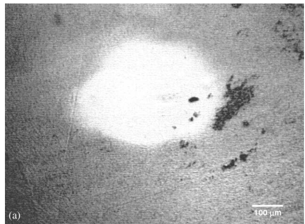
Figure 4 (a) An SEM micrographs of the multilayer condyle wear area. The high magnification micrograph at the edge of the wear area shows evidence of what appears to be thin film cracking. (b) An SEM micrograph of the multilayer fossa wear area. The high magnification micrograph shows the difference in the film texture between the as-coated and worn areas.
